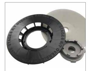
Unique CVT Oversize system from Stage6. The developers have succeeded in revising conventional systems and manufacturing a transmission consisting of forged aluminium pulleys. With these CNC-machined pulleys, a much higher degree of precision can be achieved as compared to pressed steel pulleys. The manufacturing method allows for precise angles and a defined surface roughness. At the end of the manufacturing process, a ceramic surface finish is applied to prevent abrasion and heat generation.
